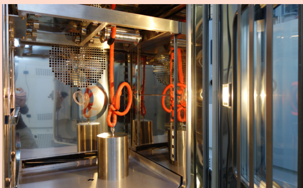
Cold Bend Cables Testing
