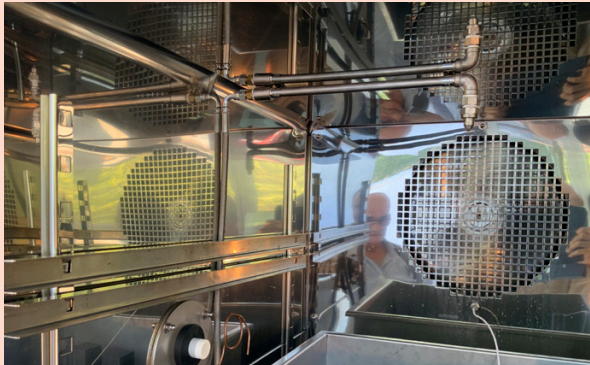
Sprinkler - Rain simulation
