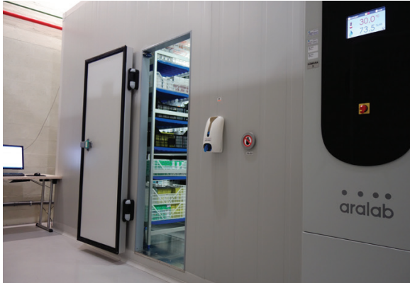
ARALAB FITOCLIMA 25.000 PH PHARMACEUTICAL PRODUCTS LONG TERM TESTING
