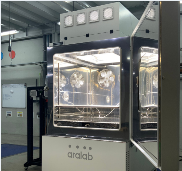
SOLAR AND UV RADIATION CHAMBER
