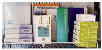
The WiFi data loggers in the drugs refrigerator immediately provide the staff with an alarm when upper or lower limit values are exceeded.
