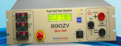
The 890ZV is an air-cooled, multi-range programmable electronic load with integrated Zero Volt Boost Supply.
