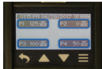
> Touch desired Preset (programmed in DataTrac Pro Software and uploaded to pump)
