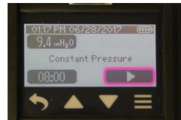
> Touch Run button in Advanced Menu to run pump in constant pressure.
