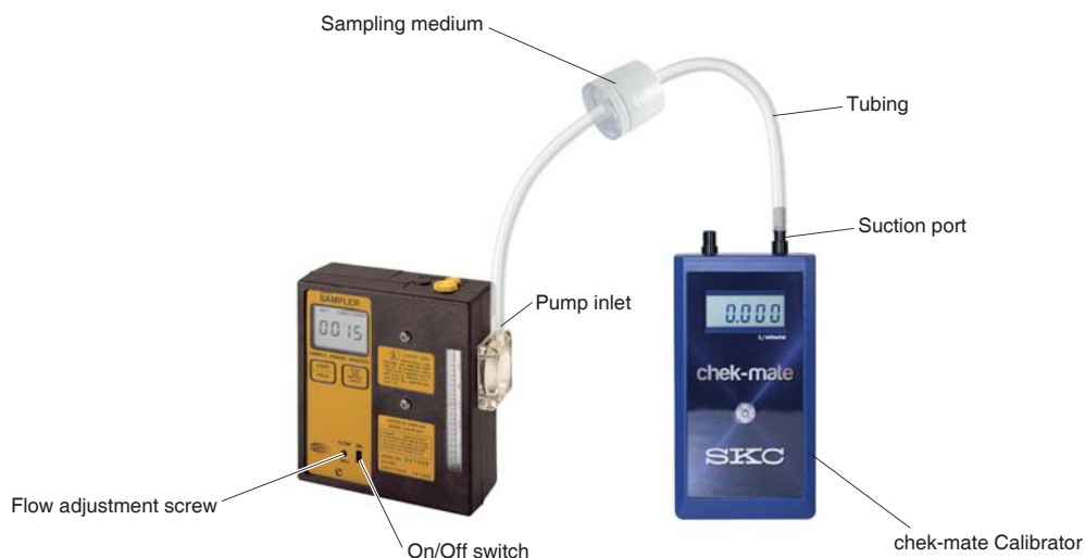
Figure 2. Calibration Train with Filter Cassette
