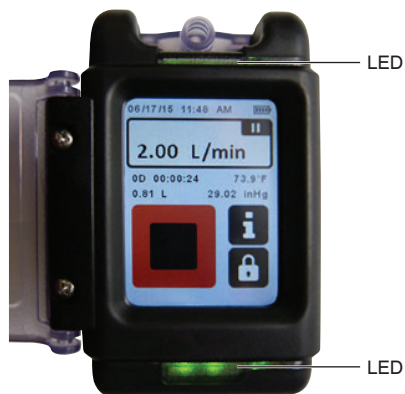
Figure 5. Green, flashing = Pump or schedule running
