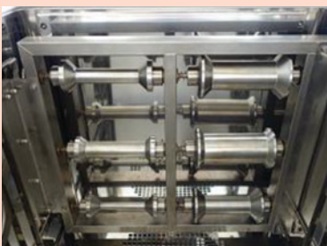
Cables/Wires winding accessory for 'Cold bend' testing
