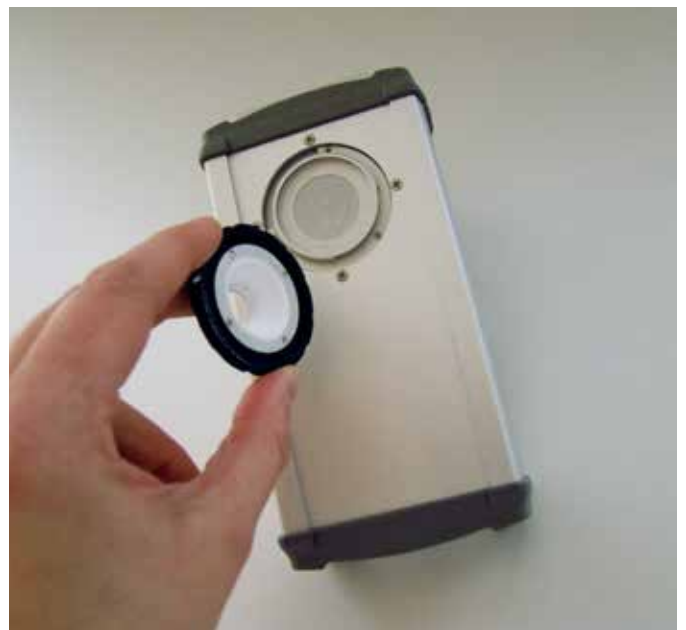
The conical measurement port is placed over the test LED and detects all the radiation in a 2pi space
