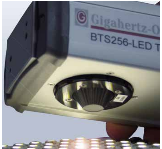
BTS256-LED for measurement of the luminous flux, spectrum, color, and color rendering index of single LEDs
