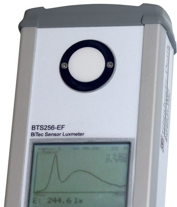
BTS256-EF for complex measurements in lighting technology, including flicker measurement
