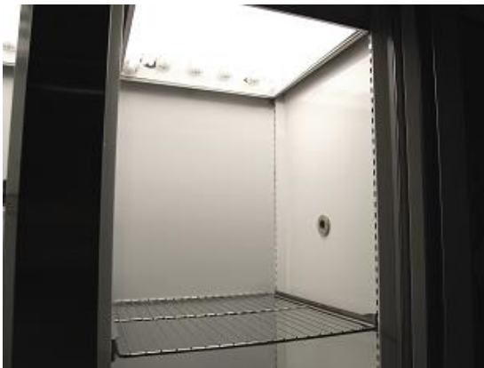
High Performance fluorescent with heat extraction system
