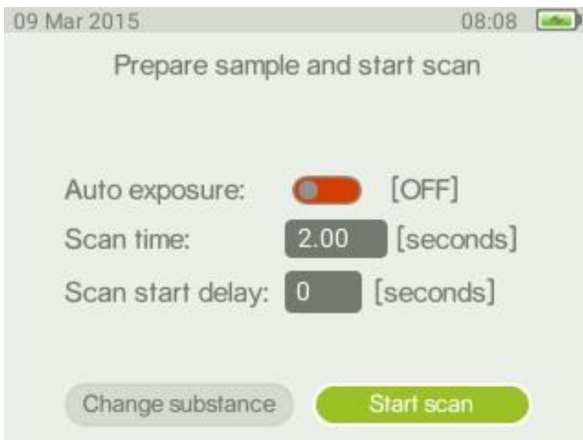
Figure 37 - Scan window with auto-exposure off
