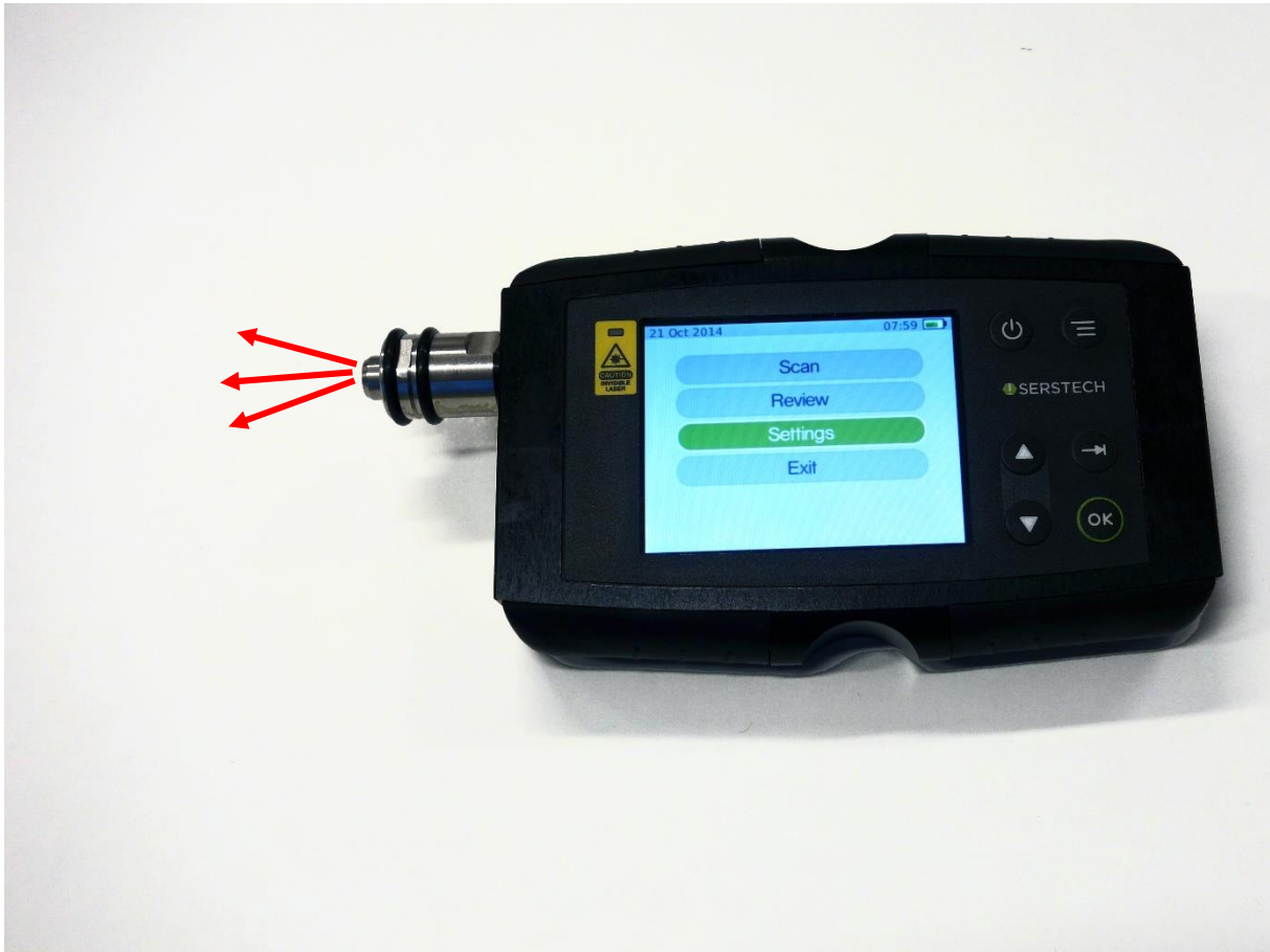
Figure 4 - Outline of the Serstech 100 Indicator. The red arrows depict the origin and direction of the laser light.
