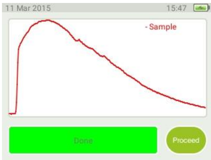
Figure 40. Spectrum flooded with fluorescence where Raman information is obscured. Not usable.
