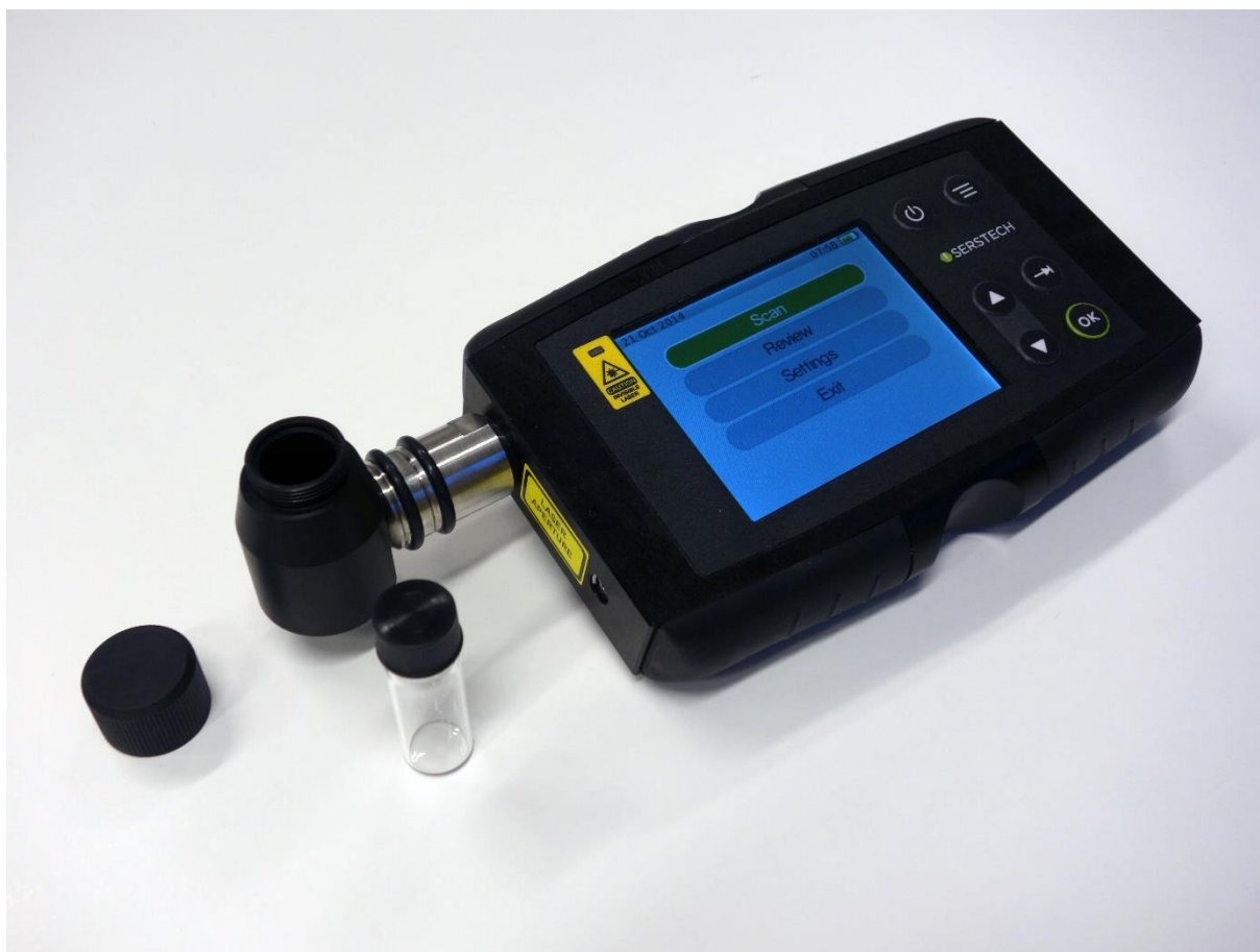
Figure 16 - Vial holder with cap and 4ml standard vial.
