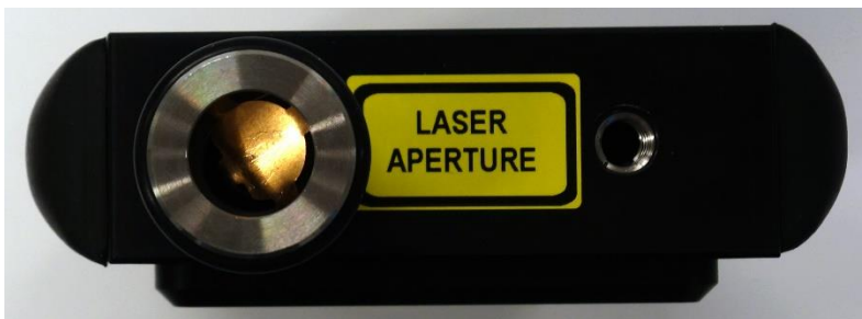
Figure 20 - Laser aperture with shutter (front view). Warning – never remove the nosepiece when the instrument is active.
