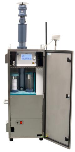
During operation, after the completion of one sampling period, a forcibly guided handling system takes a cassette with a clean filter from the storage magazine and inserts it into the sampling position. Simultaneously, the filter cassette with the dust-laden filter is removed from the sampling position and inserted into the magazine for exposed filters. The use of a Geneva drive prevents any obstructions of the complex movements of the components.
