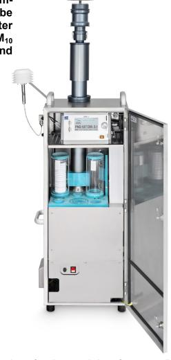
During operation, after the completion of one sampling period, a forcibly guided handling system takes a cassette with a clean filter from the storage magazine and inserts it into the sampling position. Simultaneously, the filter cassette with the dust-laden filter is removed from the sampling position and inserted into the magazine for exposed filters. The use of a Geneva drive prevents any obstructions of the complex movements of the components.
