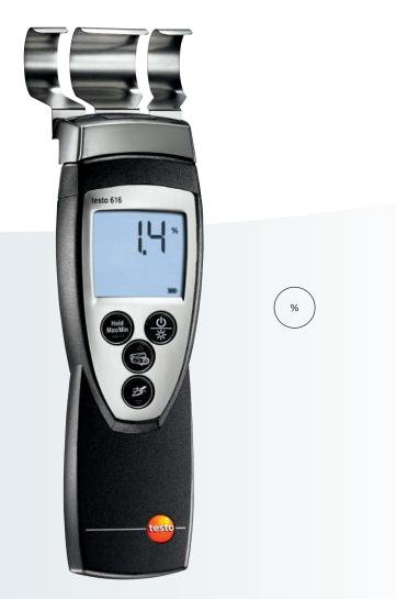
The test 616 allows fast and damage-free examination of material moisture curves in building materials and woods. It also facilitates your work in observing the drying process of floors walls and surfaces.
