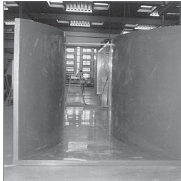
Flume for measuring surface water for the river Maas near Maastricht in the Netherlands. Customer: Waterschap Roer en Overmaas
